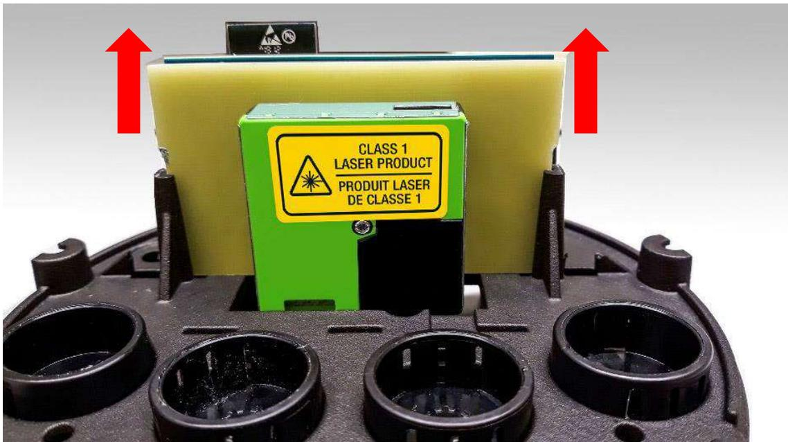
**Figure 27:** Replacing PM sensor
